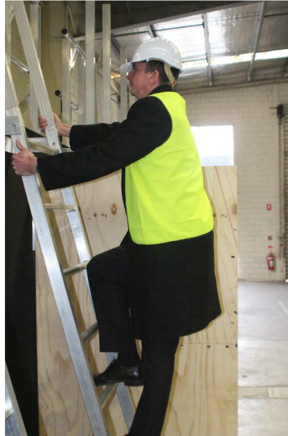
Inclined rung ladder
